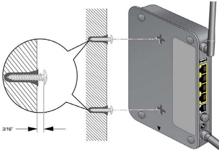
**Figure 58. Insert screws into the wall anchors**
