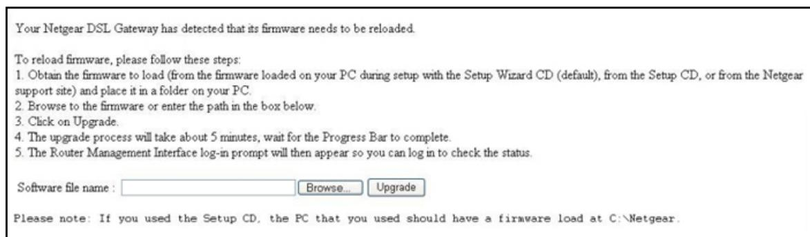
**Figure 55. Reload firmware**
