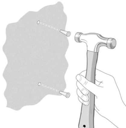
**Figure 57. Put wall anchors in the holes**
