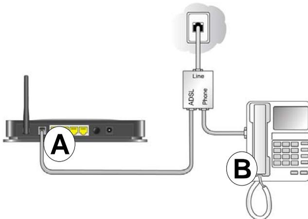
Figure 8. Cable the modem router to the microfilter
