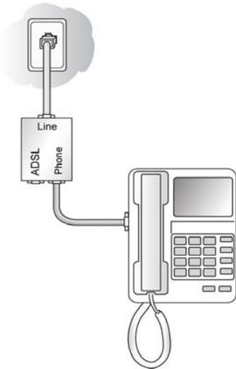
Figure 7. ADSL microfilter between phone line and phone
