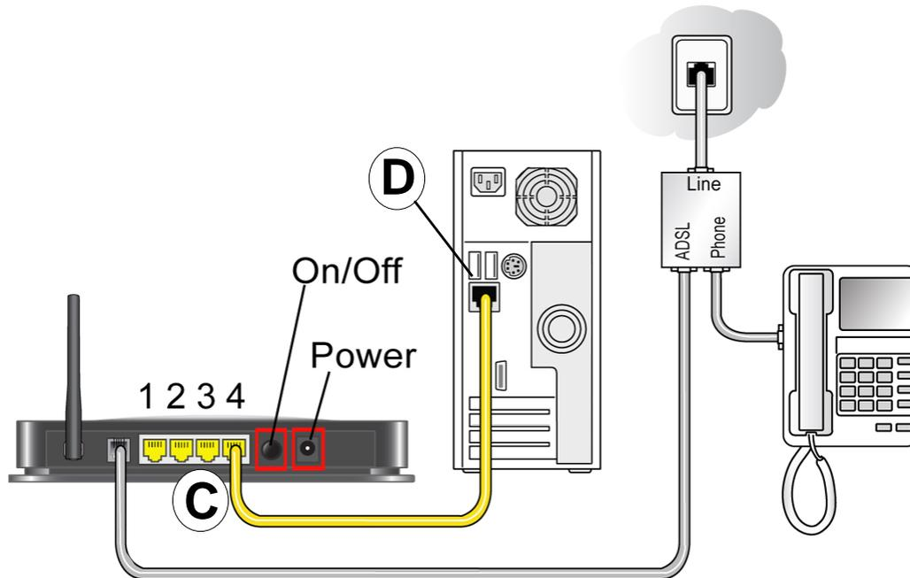
**Figure 9. Connect the Ethernet cable to your computer**
