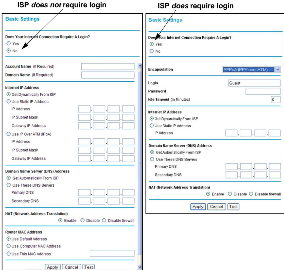
Figure 13. Basic Settings screen without (left) and with (right) login.
