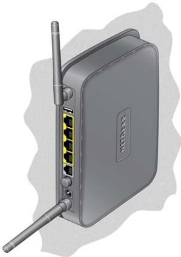
**Figure 59. Position the antennas**
