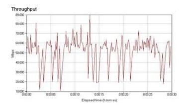
As mentioned previously, many things can impact wireless throughput, including the orientation of the client. There are three antennas in most 802.11n-equipped laptops, and in three dimensions these work (once again) a lot like rabbit ears. So I actually ran each test four times, rotating the laptop a quarter-turn for each test. The results were then averaged together.
