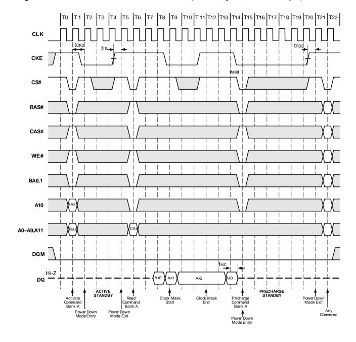
Figure 8. Power Down Mode and Clock Mask (Burst Lenght=4, CAS# Latency=2)
