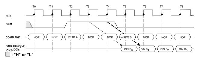
Read to Write Interval (Burst Length 3 4, CAS# Latency = 2)
