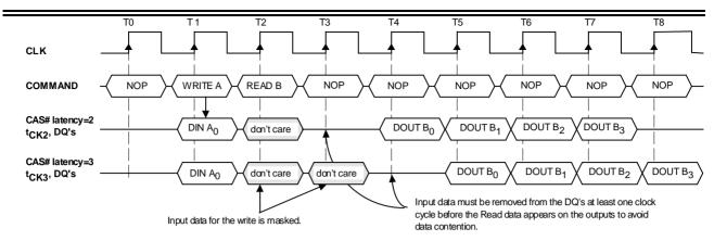
Write Interrupted by a Read (Burst Length = 4, CAS# Latency = 2, 3)
