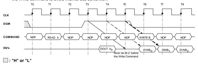
Read to Write Interval (Burst Length <sup>3</sup> 4, CAS# Latency = 3)
