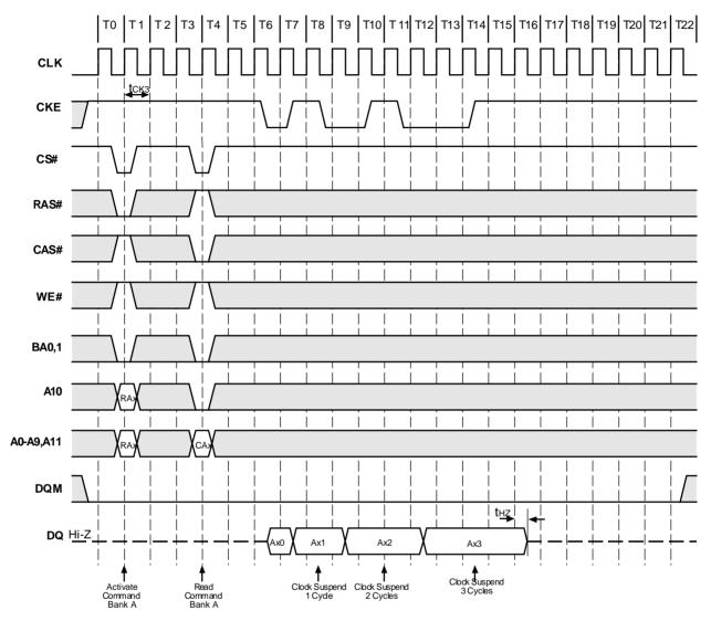
Figure 7.1. Clock Suspension During Burst Write (Using CKE)
