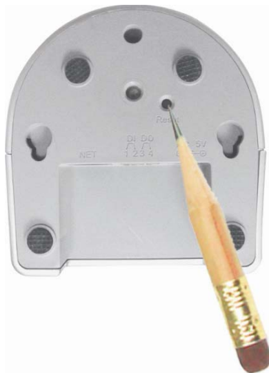
Figure 3-27: Stick on the reset button to set to the factory default
